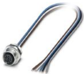
Sensor/actuator flush-type socket, 5-pos., M12, B-coded, front/screw mounting with Pg9 thread, with 0.5 m TPE litz wire, 5 x 0.34 mm 2 , stainless steel version
