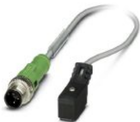
Sensor/actuator cable, 2-position, PUR, gray RAL 7001, Plug straight M12 SPEEDCON, coding: A, on Valve connector Festo ZC, with 1 LED, cable length: 0.6 m
