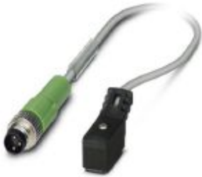
Sensor/actuator cable, 2-position, PUR, gray RAL 7001, Plug straight M8, on Valve connector Festo ZC, with 1 LED, cable length: 3 m
