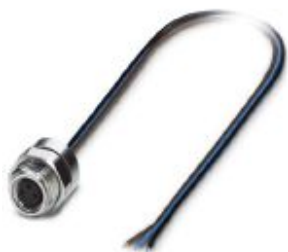
Flush-type connector, 3-position, Socket, straight, M8, Rear mounting, M12 x 1, Individual wires, cable length: 0.5 m, 0.25 mm 2 , PVC litz wire
