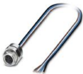
Flush-type connector, 4-position, Socket, straight, M8, Rear mounting, M12 x 1, Individual wires, cable length: 0.5 m, 0.25 mm 2 , PVC litz wire
