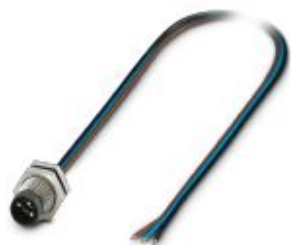
Flush-type connector, 3-position, Plug, straight, M8, Rear mounting, M8 x 1, Individual wires, cable length: 0.5 m, 0.25 mm 2 , PVC litz wire
