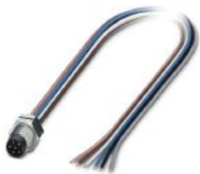
Flush-type connector, 6-position, Plug, straight, M8, Rear mounting, M8 x 1, Individual wires, cable length: 0.5 m, 0.14 mm 2 , PVC litz wire
