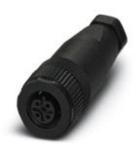
Bus system connector, 5-position, Socket straight M12, B-coded, Screw connection, knurl material: Plastic, cable gland Pg9, external cable diameter 4 mm ... 6 mm
