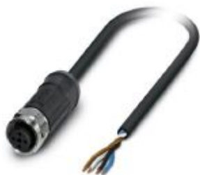
Sensor/actuator cable, 4-position, PE-X halogen-free, black-gray RAL 7021, free cable end, on Socket straight M12, coding: A, cable length: 2 m, for outdoor applications, with high-grade steel knurl
