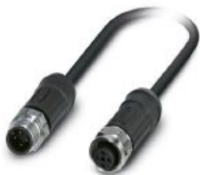
Sensor/actuator cable, 4-position, PE-X halogen-free, black-gray RAL 7021, Plug straight M12, coding: A, on Socket straight M12, coding: A, cable length: 2 m, for outdoor applications, with high-grade steel knurl
