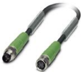
Sensor/actuator cable, 3-position, PUR halogen-free, black-gray RAL 7021, shielded, Plug straight M8, on Socket straight M8, cable length: 3 m
