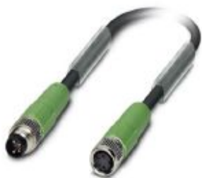
Sensor/actuator cable, 4-position, PUR halogen-free, black-gray RAL 7021, shielded, Plug straight M8, on Socket straight M8, cable length: 0.6 m
