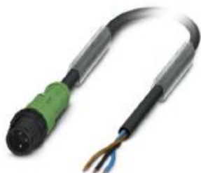
Sensor/actuator cable, 3-position, PUR halogen-free, black-gray RAL 7021, Plug straight M12, coding: A, on free cable end, cable length: 1.5 m, with plastic knurl
