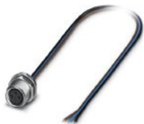
Flush-type connector, 3-position, Socket, straight, M8, Rear mounting, M10, Individual wires, cable length: 0.5 m, 0.25 mm 2 , PVC litz wire
