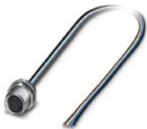
Flush-type connector, 4-position, Socket, straight, M8, Rear mounting, M10, Individual wires, cable length: 0.5 m, 0.25 mm 2 , PVC litz wire
