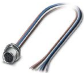
Flush-type connector, 6-position, Socket, straight, M8, Rear mounting, M10, Individual wires, cable length: 0.5 m, 0.14 mm 2 , PVC litz wire
