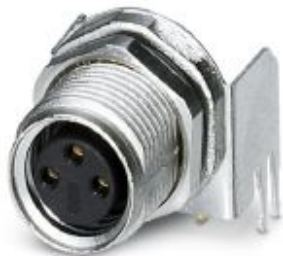
Sensor/actuator flush-type connector, socket, 3-pos. M8, rear/screw mounting with M10 fastening thread, with angled solder connection
