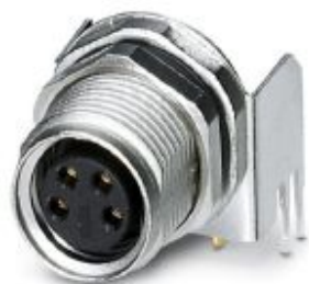
Sensor/actuator flush-type connector, socket, 4-pos. M8, rear/screw mounting with M10 fastening thread, with angled solder connection
