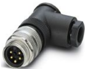
Connector, Universal, 5-position, Plug angled 7/8"-UNF, Coding: A, Screw connection, knurl material: Zinc die-cast, nickel-plated, cable gland Pg11, external cable diameter 8 mm ... 10 mm, Contact 3 capacitive
