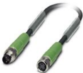
Sensor/actuator cable, 3-position, PUR halogen-free, black-gray RAL 7021, shielded, Plug straight M8, on Socket straight M8, cable length: 0.3 m
