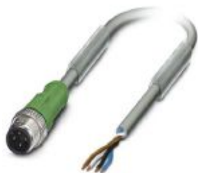
Sensor/actuator cable, 4-position, PUR halogen-free, resistant to welding sparks, highly flexible, gray RAL 7001, Plug straight M12, coding: A, on free cable end, cable length: 10 m, for robots and drag chains
