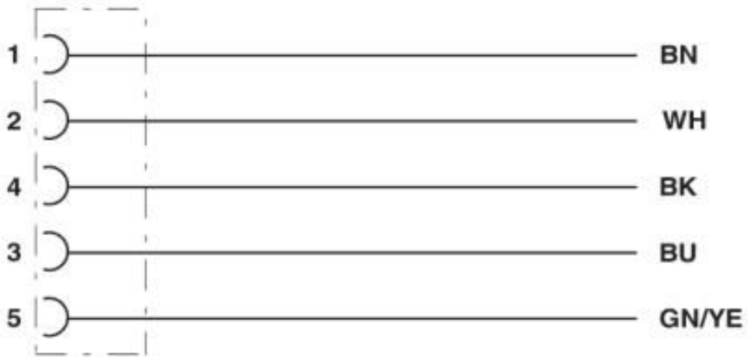
Contact assignment of the M12 sockets
