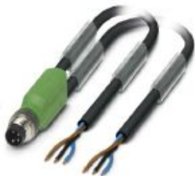
Sensor/actuator cable, 3-position, PUR halogen-free, black-gray RAL 7021, Plug straight M8, on free cable end and free cable end, cable length: 10 m
