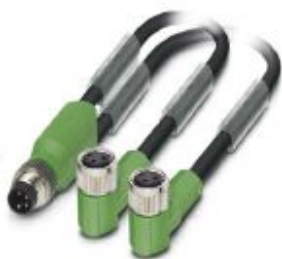
Sensor/actuator cable, 3-position, PUR halogen-free, black-gray RAL 7021, Plug straight M8, on Socket angled M8 and Socket angled M8, cable length: 0.3 m
