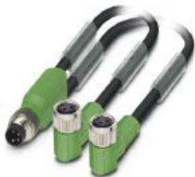
Sensor/actuator cable, 3-position, PUR halogen-free, black-gray RAL 7021, Plug straight M8, on Socket angled M8 and Socket angled M8, cable length: 3 m
