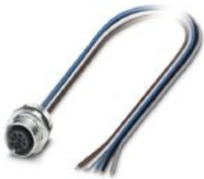
Sensor/actuator flush-type socket, 5-pos. M12, A-coded, front/screw mounting with M16 thread, with 0.5 m TPE litz wire, 5 x 0.34 mm 2 , stainless steel version
