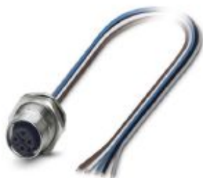
Panel feed-through, Universal, 5-position, Socket, straight, M12-SPEEDCON, A-coded, Rear mounting, Pg9, cable length: 1 m, 0.34 mm 2 , TPE litz wire
