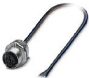
Flush-type connector, Universal, 3-position, Socket, straight, M12-SPEEDCON, A-coded, Front mounting, M16 x 1.5, Individual wires, cable length: 0.5 m, 0.34 mm 2 , TPE litz wire
