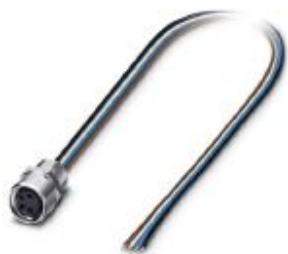
Flush-type connector, 4-position, Socket, straight, M8, Front mounting, M8 x 0.5, Individual wires, cable length: 0.5 m, 0.25 mm 2 , PVC litz wire
