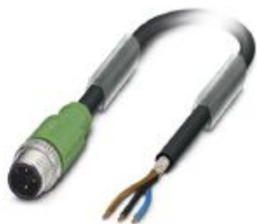
Sensor/actuator cable, 3-position, PUR halogen-free, black-gray RAL 7021, shielded, Plug straight M12, coding: A, on free cable end, cable length: 10 m
