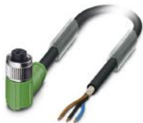
Sensor/actuator cable, 3-position, PUR halogen-free, black-gray RAL 7021, shielded, free cable end, on Socket angled M12, coding: A, cable length: 10 m
