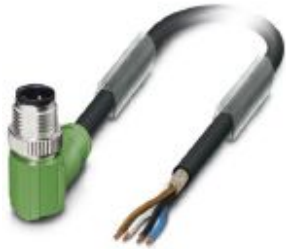
Sensor/actuator cable, 4-position, PUR halogen-free, black-gray RAL 7021, shielded, Plug angled M12, coding: A, on free cable end, cable length: 10 m
