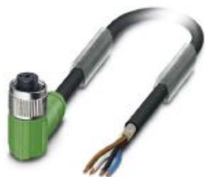
Sensor/actuator cable, 4-position, PUR halogen-free, black-gray RAL 7021, shielded, free cable end, on Socket angled M12, coding: A, cable length: 10 m
