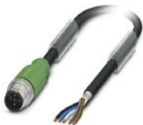
Sensor/actuator cable, 5-position, PUR halogen-free, black-gray RAL 7021, shielded, Plug straight M12, coding: A, on free cable end, cable length: 10 m
