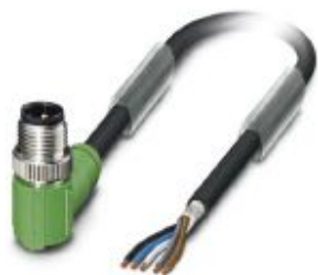
Sensor/actuator cable, 5-position, PUR halogen-free, black-gray RAL 7021, shielded, Plug angled M12, coding: A, on free cable end, cable length: 10 m
