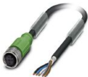
Sensor/actuator cable, 5-position, PUR halogen-free, black-gray RAL 7021, shielded, free cable end, on Socket straight M12, coding: A, cable length: 10 m
