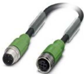
Sensor/actuator cable, 3-position, PUR halogen-free, black-gray RAL 7021, shielded, Plug straight M12, coding: A, on Socket straight M12, coding: A, cable length: 0.6 m
