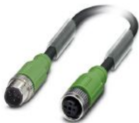
Sensor/actuator cable, 4-position, PUR halogen-free, black-gray RAL 7021, shielded, Plug straight M12, coding: A, on Socket straight M12, coding: A, cable length: 3 m
