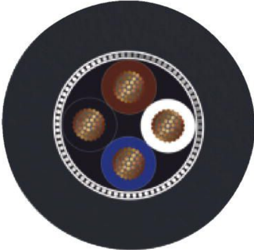
Cable cross section
