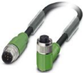
Sensor/actuator cable, 5-position, PUR halogen-free, black-gray RAL 7021, shielded, Plug straight M12, coding: A, on Socket angled M12, coding: A, cable length: 0.6 m
