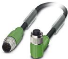
Sensor/actuator cable, 5-position, PUR halogen-free, black-gray RAL 7021, shielded, Plug straight M12, coding: A, on Socket angled M12, coding: A, cable length: 1.5 m
