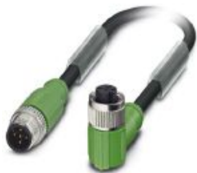
Sensor/actuator cable, 5-position, PUR halogen-free, black-gray RAL 7021, shielded, Plug straight M12, coding: A, on Socket angled M12, coding: A, cable length: 3 m
