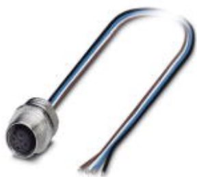
Sensor/Actuator flush-type socket, 4-pos., M12, A-coded, front/screw mounting with Pg9 thread, with 1 m TPE litz wire, 4 x 0.25 mm 2
