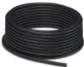
Master cable for sensor/actuator boxes, with PE conductor, unshielded, material PUR/PVC, 11-pos., 8 x 0.34 mm 2 and 3 x 0.75 mm 2
