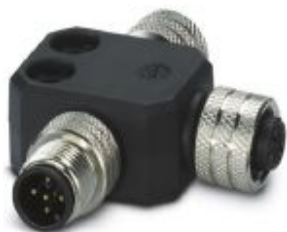
T distributor, CANopen®, DeviceNet™, 5-position, Plug straight M12, coding: A, on Socket straight M12, coding: A and Socket straight M12, coding: A
