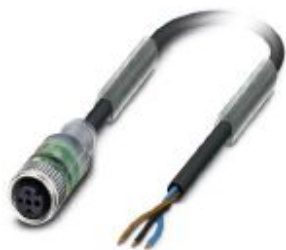
Sensor/actuator cable, 3-position, PVC, black RAL 9005, free cable end, on Socket straight M12, coding: A, with 2 LEDs, cable length: 5 m
