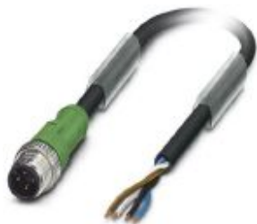
Sensor/actuator cable, 4-position, PUR, black-gray RAL 7021, Plug straight M12, coding: A, on free cable end, cable length: 15 m
