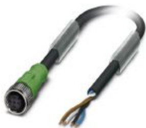
Sensor/actuator cable, 4-position, PUR, black-gray RAL 7021, free cable end, on Socket straight M12, coding: A, cable length: 15 m
