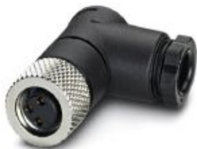
Connector, Universal, 4-position, Socket angled M8, Coding: A, Solder connection, knurl material: Nickel-plated brass, external cable diameter 3.5 mm ... 5 mm
