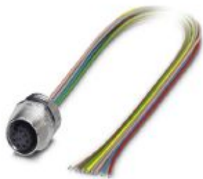
Sensor/Actuator flush-type socket, 8-pos., M12, A-coded, front/screw mounting with Pg9 thread, with 0.5 m TPE litz wire, 8x 0.25 mm 2
