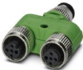
Y distributor, 4-position, unshielded, Plug straight M12, coding: A, on Socket straight M12, coding: A, PIN 2+4 bridged and Socket straight M12, coding: A, PIN 2+4 bridged
